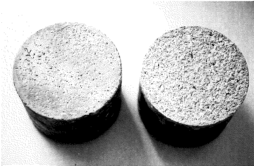
Figure 2: surface after the freeze - thaw tests in salty solution.
